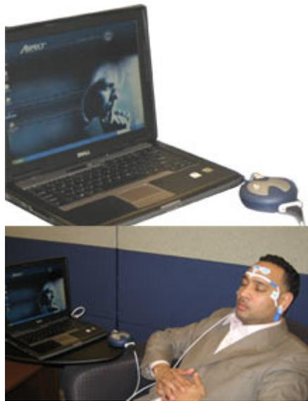
Mind reading: The system above was used to predict whether patients should be kept on one antidepressant or switched to another. The strap around the subject's head contains electrodes that pick up brain waves. The strap hooks up to a hockey-puck-size device that digitizes and filters the EEG signal before sending it on to a laptop for processing.
